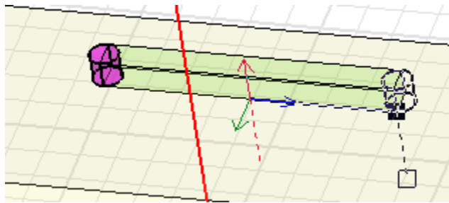
Figure 13: Duplicated cylinder with the mid point of the slot as the reference
