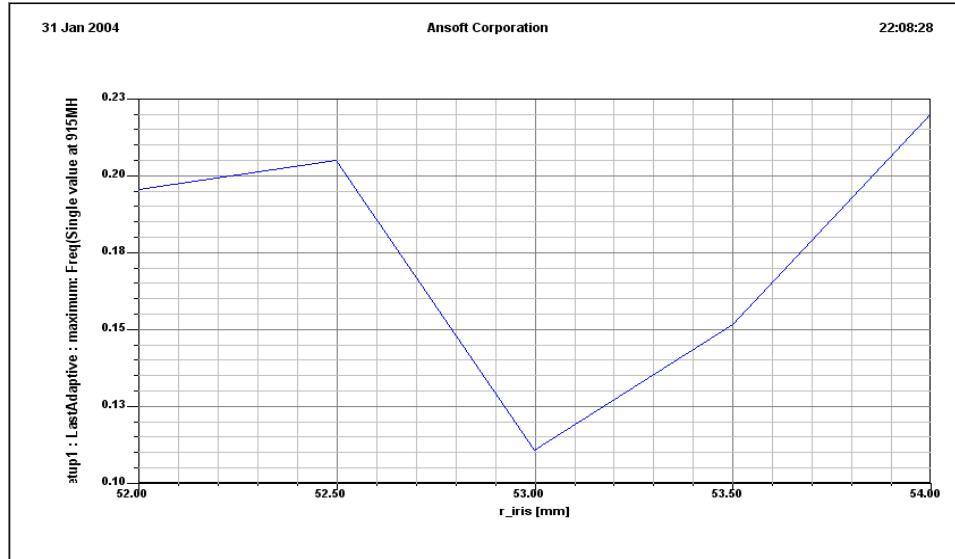
According to the graph, minimum reflection occurs at approximately 5.3cm. This should produce optimal power transfer into the cavity. With this information, redefine the “r\_iris” variable under HFSS -> Design Variables. Follow all previously completed steps in this tutorial and rerun the Analysis with the new variable definition. Create Reports and generate S11 plot. What can you determine from the new plot ?
