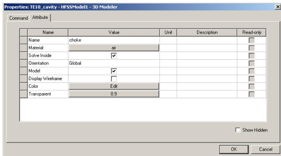
Click OK when complete. Step one of the “choke” is complete and should appear as follows:
