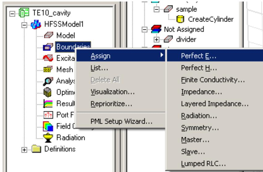
Name the boundary “PEC1”. Follow the same procedure and assign the “divider” as “PEC2”. All surfaces of the resonating geometry are now defined.
