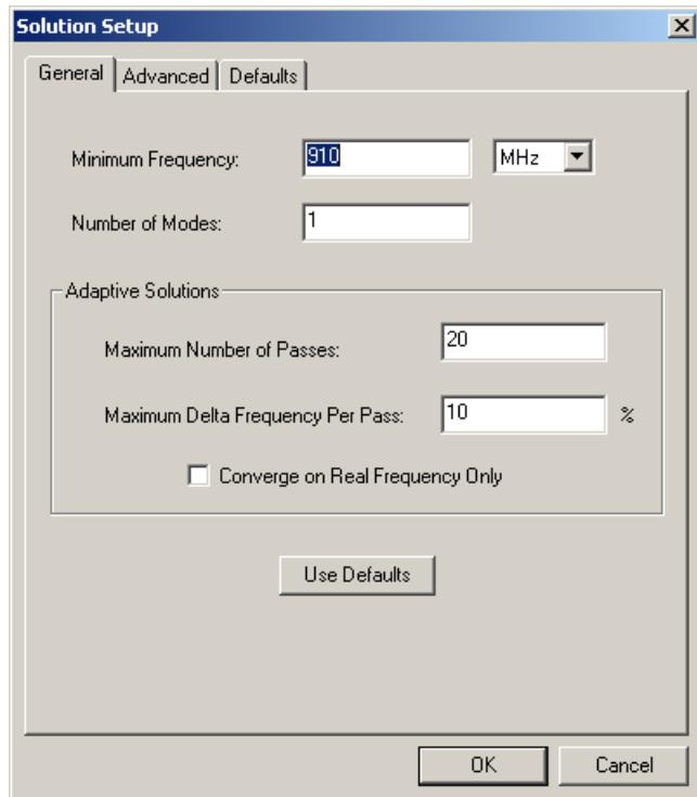
The eigenmode solution will find the cavity resonance and the Q of the cavity. Run the Validation Check as in the previous example to verify correct setup. Run the Analysis. When complete, right-click **Setup1-> EigenmodeData**.
