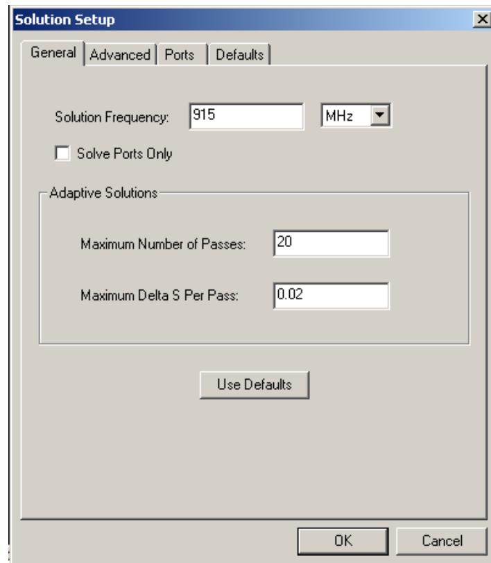
If simulation time is excessive, the user can lessen the computational load by allowing Maximum Delta S  $\geq .05$ .
