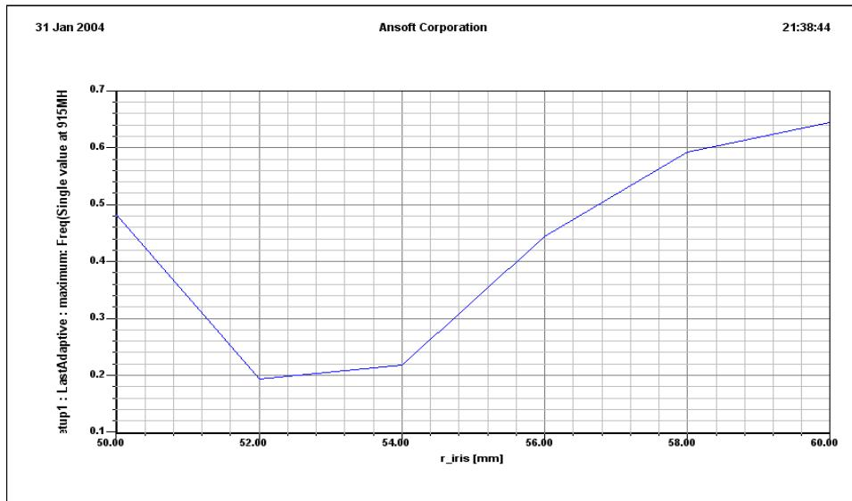
The above figure displays  $S_{11}$  vs. iris radius. We find that minimum reflection occurs between 5.2cm and 5.4cm. With this information, we can now re-analyze the iris variable defined from 5.2cm to 5.4cm. Set the step size to .05cm. Follow all previous step and re-analyze with the new settings.
