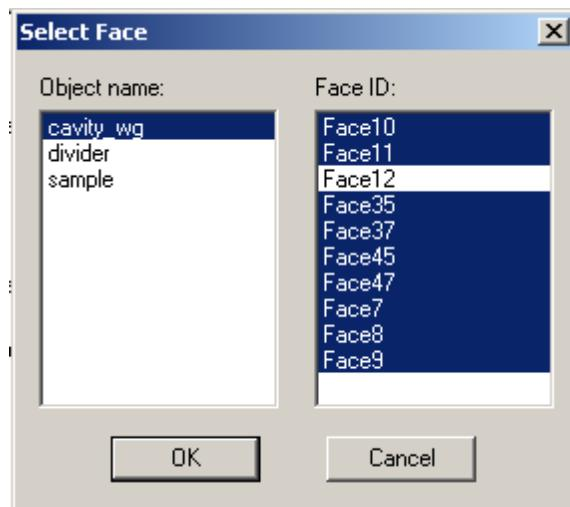
Notice that “Face12” has not been highlighted. The excitation source will be defined in the next section. This face is used for the source.
