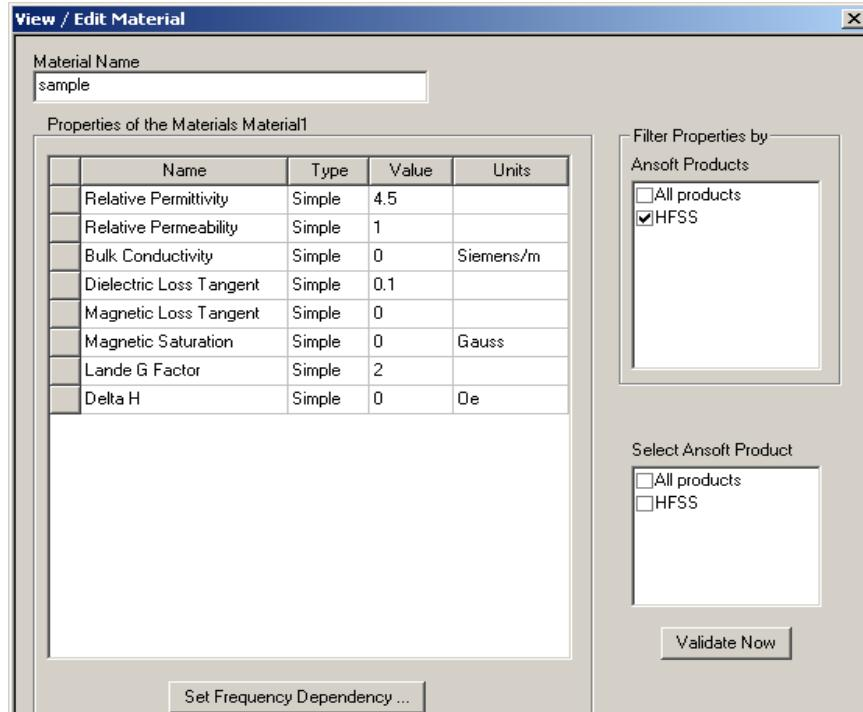
The material is defined as complex by defining the dielectric loss tangent. See help for further explanation of complex material assignment.
