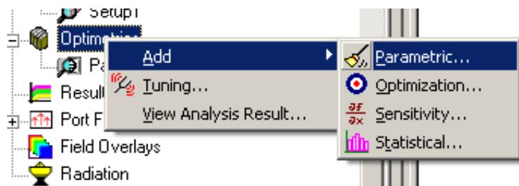
Select "r\_iris" as the variable. The radius will begin at 5cm and end at 6cm with a step size of .2cm. Click Add and OK when finished.
