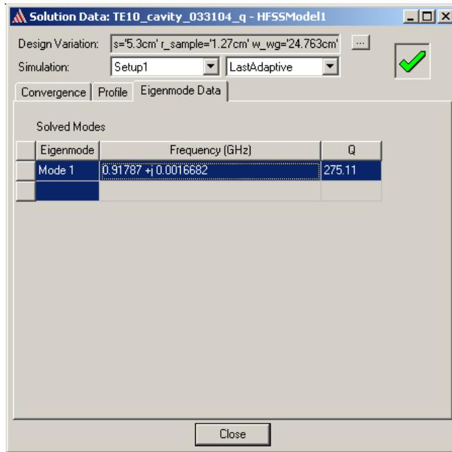
The Eigenmode solution found the resonant frequency at 917MHz. This calculation could be made more accurate by decreasing the Maximum Delta Frequency Per Pass within the analysis setup.
