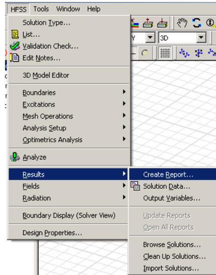
The S-parameter plot will display the reflection coefficient vs. frequency. The resonant frequency can be visually determined from the plot. Enter the following:
