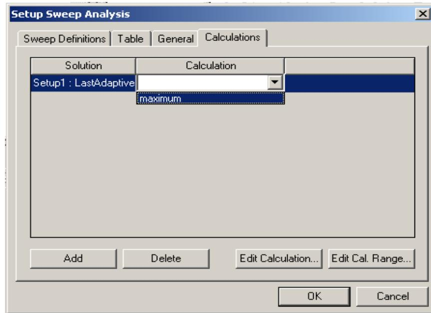
Click **OK** when complete. From the project tree, right-click **Optimetrics**  $\Rightarrow$  **Analyze**. Depending on the machine, analysis can take from 5 minutes to 1 hour.
