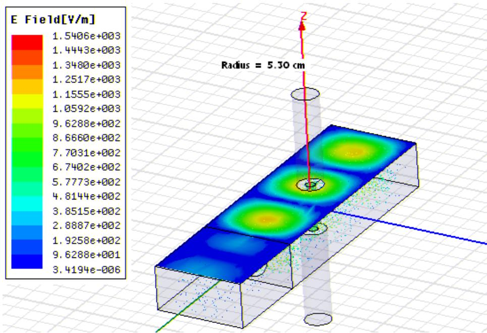
Optimetrics should be used from this point to re-optimize the iris for maximum power transfer. This will be left as an exercise for the user.
