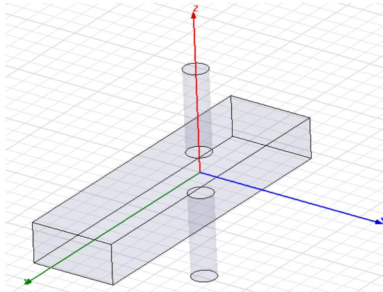
In the next step, the “sample” structure is created. A custom material, with a complex dielectric constant, will be defined. Begin by selecting Draw Cylinder from the 3D toolbar. From the property window, select the following:
