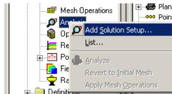
The cavity is expected to resonate at a frequency of 915MHz. Enter this as the solution frequency. Set Maximum Number of Passes to 20 and Delta S to .02.
