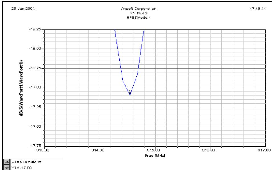
The resolution in this analysis is a limiting factor. Resolution is increased by narrowing the sweep range and keep the count size constant. The user can also explore other types of sweeps (see Ansoft help).
