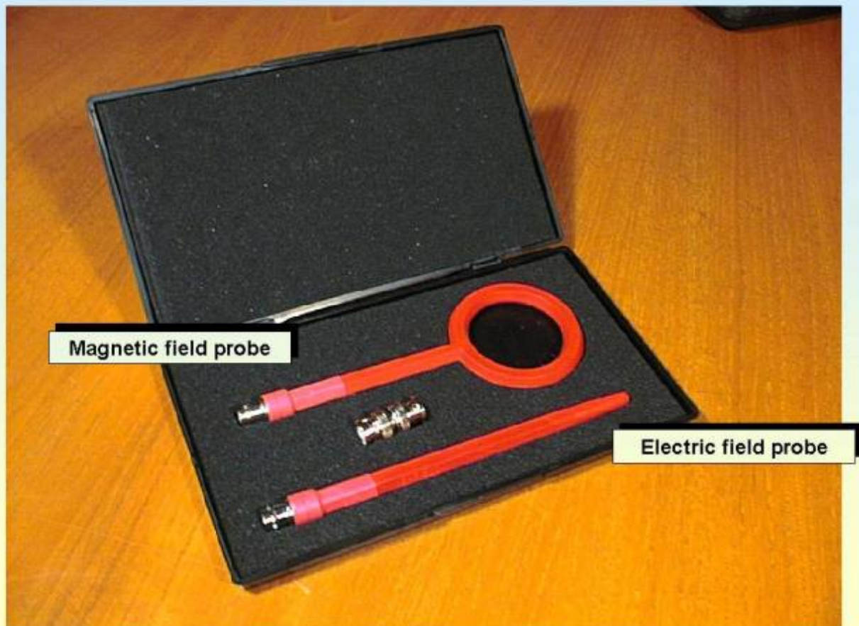
Figure 3 Example of a proprietary close-field probe set
