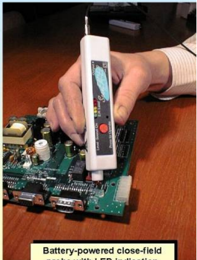
Figure 6 Two examples of 'bug detectors'
