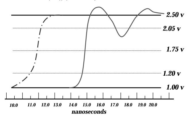
$V_{il^-max} = 1.20V$ ,  $V_{ih^-min} = 2.05V$ ,  $V_{ref^-Driver} = 1.75 V$ ,  $V_{steady^-state-high} = 2.50 V$ ,  $V_{steady^-state-low} = 1.0V$
