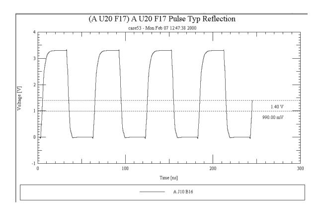
$V_{il^-max} = 0.7V, \quad V_{ih^-min} = 2.55V, \quad V_{ref^-Driver} = 1.75~V, \quad V_{steady^-state-high} = 3.30~V, \quad V_{steady^-state-low} = 0.0V$
