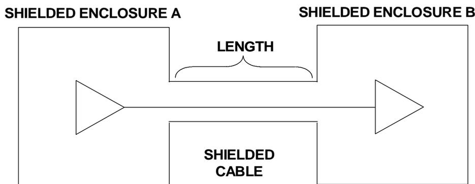
FULLY SHIELDED ENCLOSURES CONNECTED BY FULLY SHIELDED CABLE KEEP ALL INTERNAL CIRCUITS AND SIGNAL LINES INSIDE THE SHIELD.
