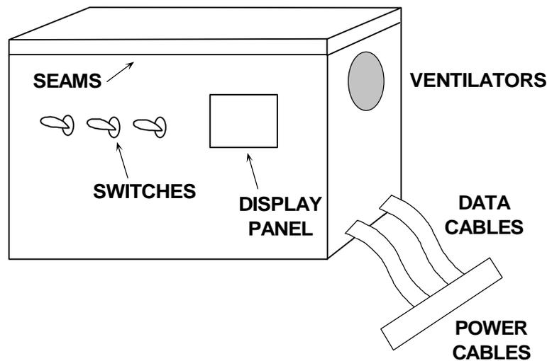
The longest dimension (not the total area) of an opening is used to evaluate the ability of external fields to enter the enclosure, because the openings behave as slot antennas. Equation 7.10 can be used to calculate the shielding effectiveness, or the susceptibility to EMI leakage or penetration, of an opening in an enclosure:
