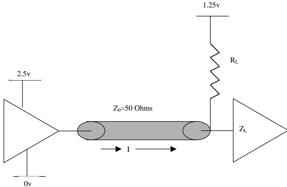
(a) Assume:  $R_{oH} = 15 \text{ Ohms}$ ,  $R_{oL} = 25 \text{ Ohms}$ ,  $Z_0$  of T-Line = 50 Ohms,  $Z_L = \infty$ ,  $R_L = \infty$ , **FALLING EDGE** waveform. **(30 points)**
