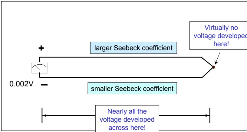
Perhaps the most misunderstood issue regarding thermocouples is that no voltage is produced at the measurement junction. The junction completes the circuit so that current flow can take place. A voltage is developed along each wire as the temperature changes. The voltage difference is observed at the receiving end because the two differing metals have different Seebeck coefficients and produce a voltage difference at the meter point.
