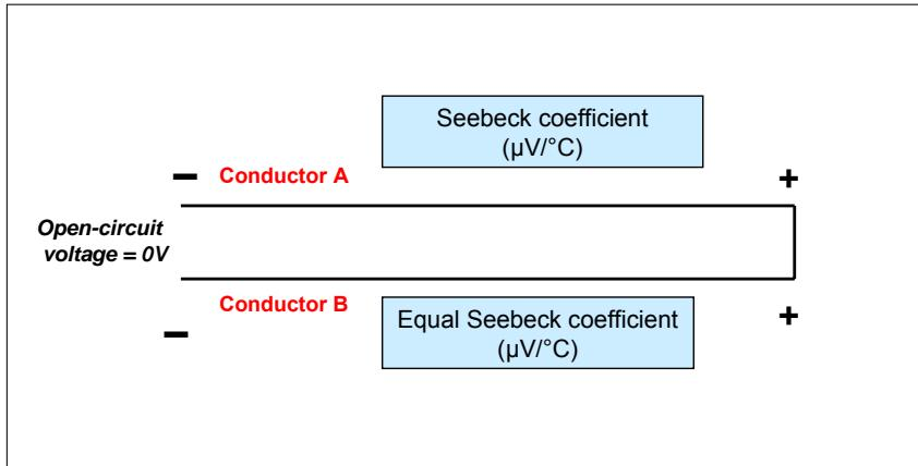
Direct measurement of the Seebeck voltage of a single wire is impossible. Another wire of the same metal produces an identical Seebeck voltage resulting in a net voltage of 0V at the measurement points.
