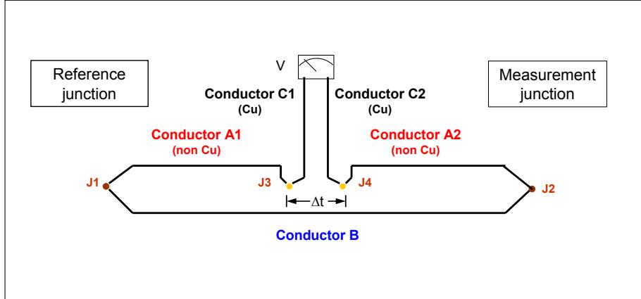
A copper-to-copper connection is unique to the case of the “type T” thermocouple. But when a thermocouple other than the “type T” is employed parasitic thermocouples are created at the meter connections or leads leading to the meter function. These parasitic thermocouples may introduce measurement errors. Each generates a Seebeck voltage dependent on the junction materials and relevant temperature gradient.
