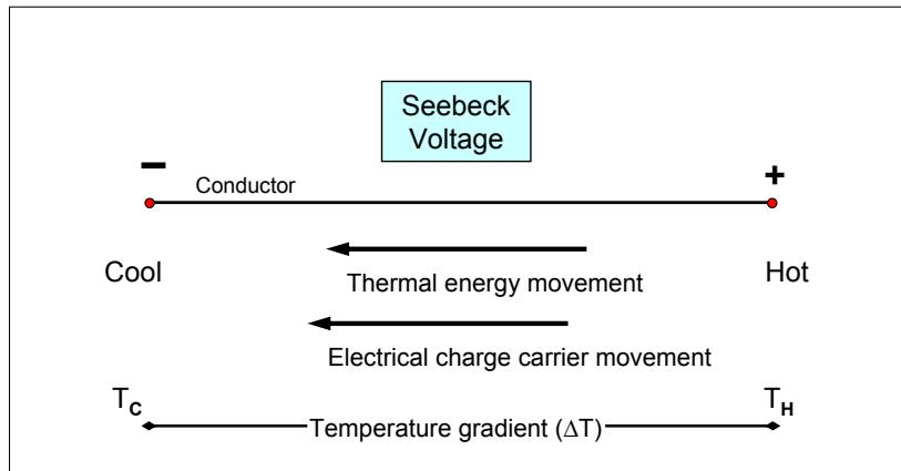
A simple wire of any metal will produce a voltage when there is a temperature difference between the two ends. Yes... believe it.
