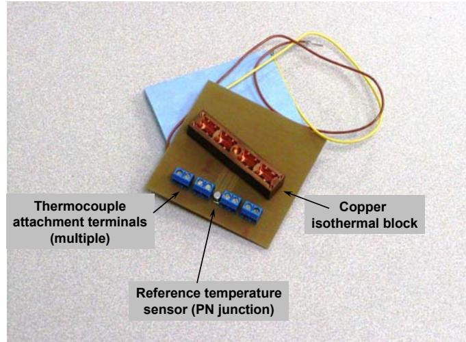
This is an image of an isothermal block that is intended for 4 individual thermocouples. The copper isothermal block fits over plastic terminal blocks. It has sufficient thermal mass such that all of the terminals should be held very close in temperature.
