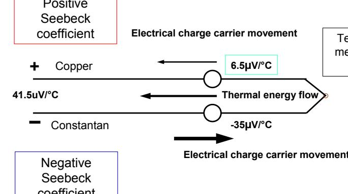
Different thermocouple materials have different capacities for moving charge carriers in response to thermal flow. The current level in one conductor will overcome or complement the potential for thermally generated current flow in the other conductor. The result is a continuous current flow that is the difference between the currents generated in the two conductors.
