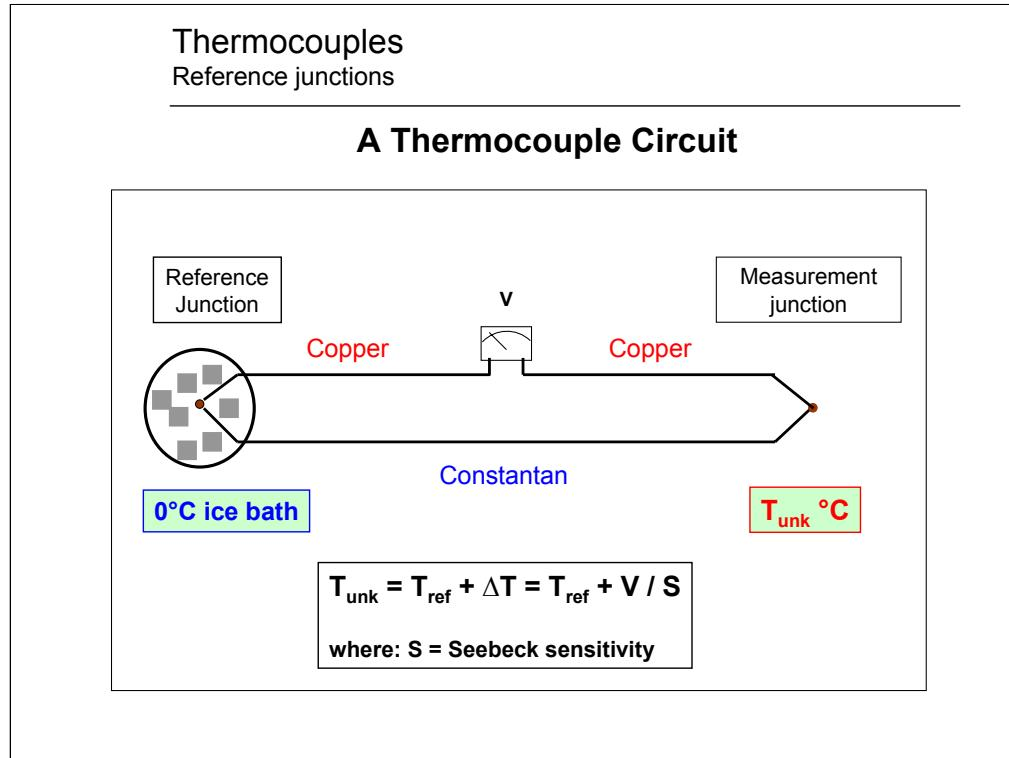
Placing the reference junction in an ice bath with a temperature very close to 0°C allows for the unknown temperature to be determined using the following relations:
