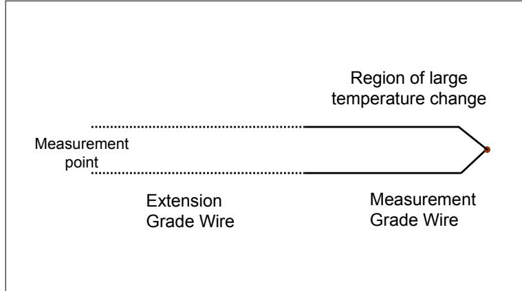
One way to avoid the problems associated with creating parasitic thermocouple junctions is to use extension wires similar in characteristics to the actual thermocouple section.
