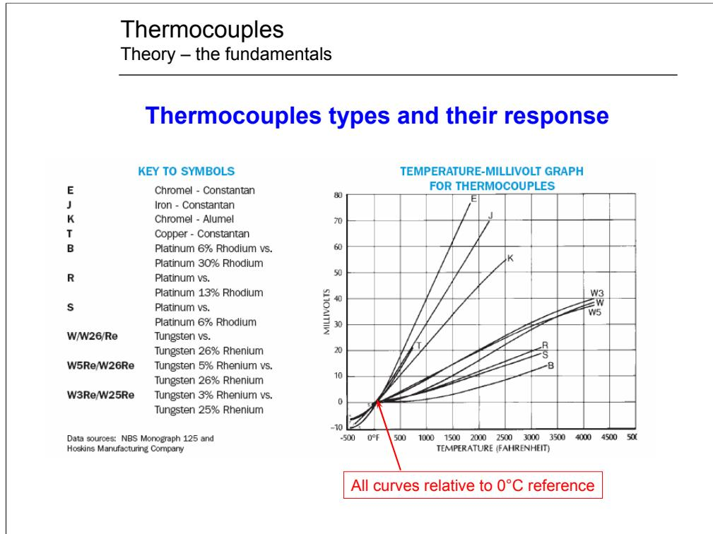
Thermocouples are classified by type which is associated with their useable temperature range, sensitivity and accuracy. The commonly used metals include: chromium, copper, nickel, iron, platinum, rhodium, and rhenium.
