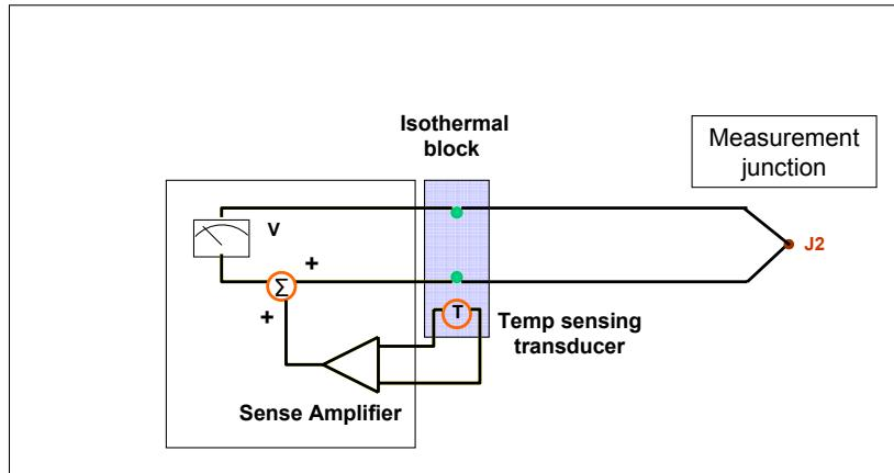
In a practical hardware compensation scheme the secondary transducer's voltage is appropriately gained and summed within the measurement circuit's path. The secondary temperature sensing transducer is mounted to the isothermal block. This can be a thermistor, RTD etc. Its resistance tracks the temperature of the isothermal block and is converted by the sense amplifier to a voltage that is summed or subtracted at the summing junction.
