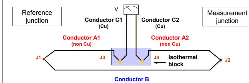
With the “type T” thermocouple the copper line can be opened and directly connected to copper extension lines without forming parasitic thermocouples. But with other materials that won’t be the case. Even then it’s not the end of the world because the two parasitic junctions, J3 and J4, will produce equal and opposite voltages - provided they are identical and at the same temperature. Moderately accurate measurements will be obtained even if they aren’t.
