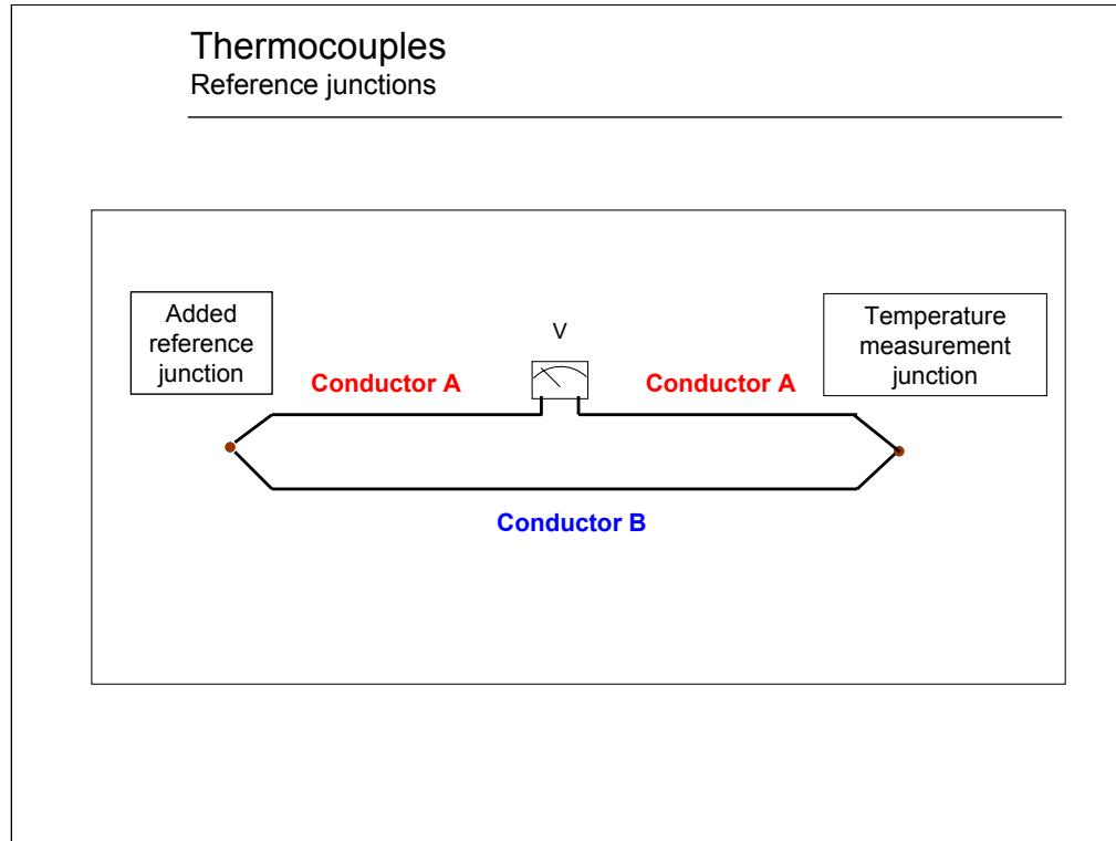
The thermocouple example in the previous slide had a thermoelectric sensitivity of about  $41.5\mu\text{V}/^\circ\text{C}$ . That is an important bit of information, but equally important and missing is a temperature reference point. A temperature change can be measured, but the actual temperature is still an unknown. Adding a second junction and holding it at a known reference temperature allows an unknown temperature at the other junction to be found.
