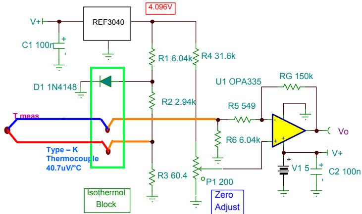
This is a complete thermocouple amplifier for a type K thermocouple. It features an OPA335 CMOS, zero-drift op-amp and includes cold junction compensation (isothermal block) and incorporates a diode thermal sensing circuit for hardware compensation.
