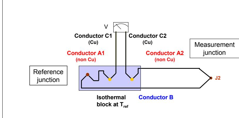
Often it is not practical to include an ice bath reference as part of the measurement system. Shown here the reference junction has now been located at the isothermal block along with the parasitic junctions. As long as the parasitic junctions are held at a common temperature they will cancel each other's Seebeck voltage contribution.
