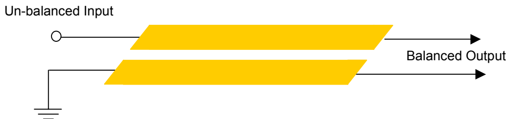
Figure 6 Simple coupled line balun
