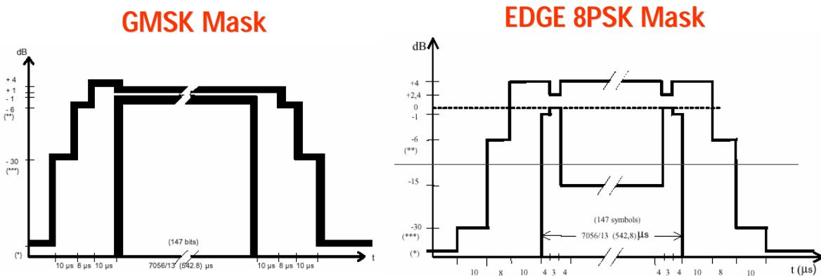
The amplitude modulation in EDGE requires that a different power versus time mask be used.
