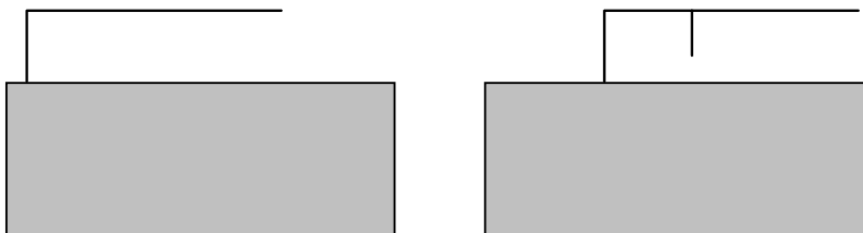
Figure 7. Tilted Whip and F - Antenna (Note the Ground Plane Area)
