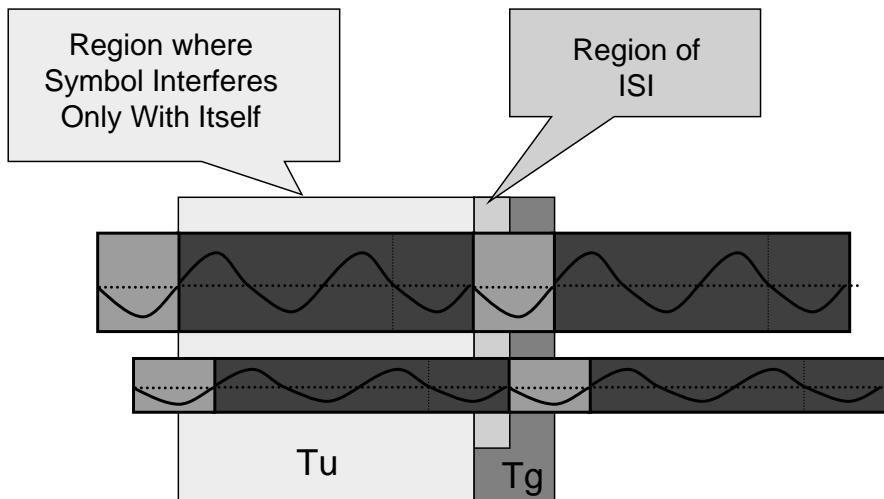
This drawing illustrates how the addition of a guard interval helps with ISI. Shown are two copies of the same signal. Each copy took a different path so they will arrive at the receiver at slightly different times where they will be combined in the receiver's antenna into a single signal. In the time interval denoted by the yellow box marked  $T_u$ , the signal will only interfere with itself. This amounts to a scaling and rotation of the symbol, nothing more.
