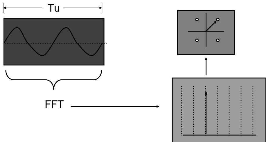
At the receiver, ignoring channel affects, the time waveform is digitized and an then converted back to a symbol using an FFT.
