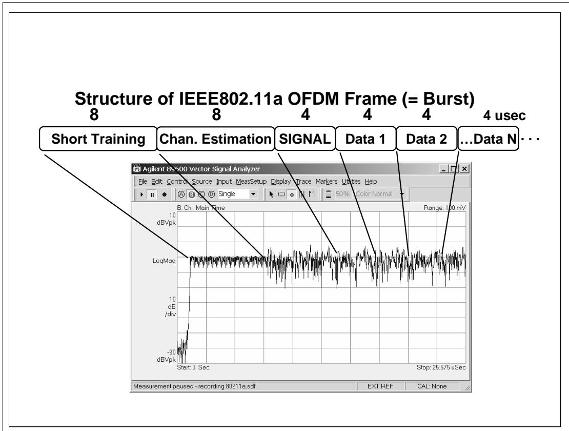
Looking at the structure of an 802.11a burst, there are three sections to every frame (a frame is an RF burst, and consists of multiple symbols):
