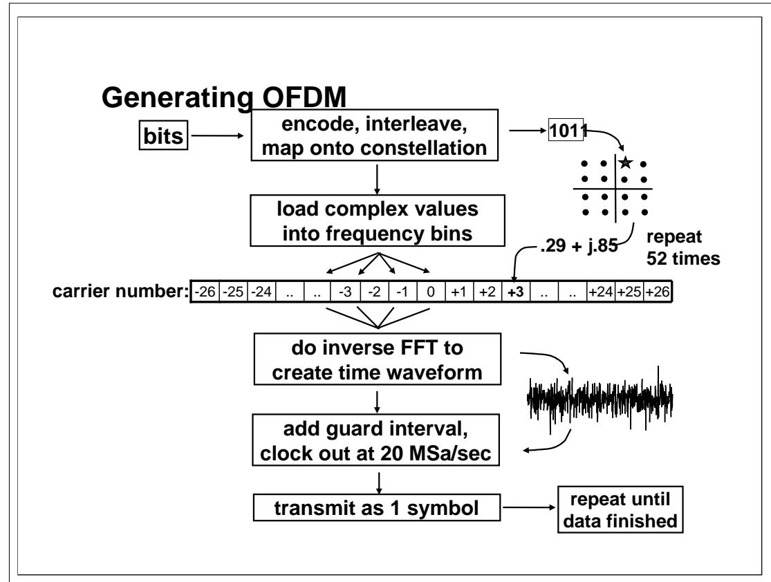
Generation of OFDM signals tends to require high performance DSP engines. The steps include:
