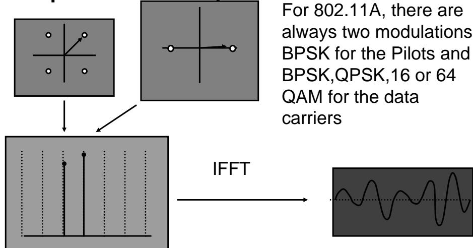
For 802.11A, there are always two modulations: BPSK for the Pilots and BPSK, QPSK, 16 or 64 QAM for the data carriers
