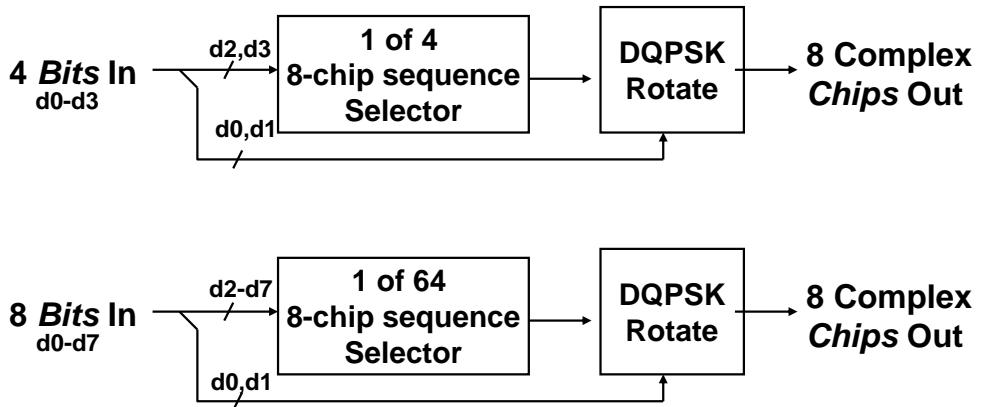
To achieve 5.5 and 11 MBit/sec rates, the spreading length is first reduced from 11 to 8. This increases the symbol rate from 1 Msym/sec to 1.375 Msym/sec. To achieve 5.5 MBit/sec bit rates with 1.375 MHz symbol rates we need to transmit 5.5/1.375 or 4 bits/symbol. For 11 MBit/sec we obviously need 8 bits/symbol
