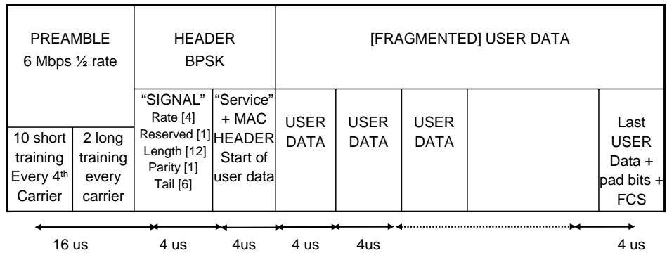
A WLAN device only transmits or receives at one point in time. Transmissions occur as bursts [frames] which vary in length and spacing, usually in the range of a few hundred microseconds to one millisecond. The 802.11b CCA receiver test draws attention to the longest possible 5.5Mbps frame being 3.65ms.
