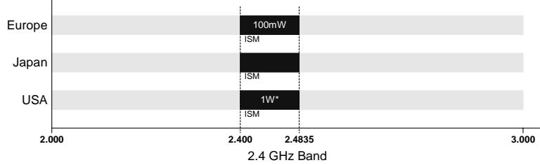
\*Per FCC 00-312, CFR 47 part 15 amended to allow 1W divided by BW in MHz (e.g. 5 MHz = 200mW)
