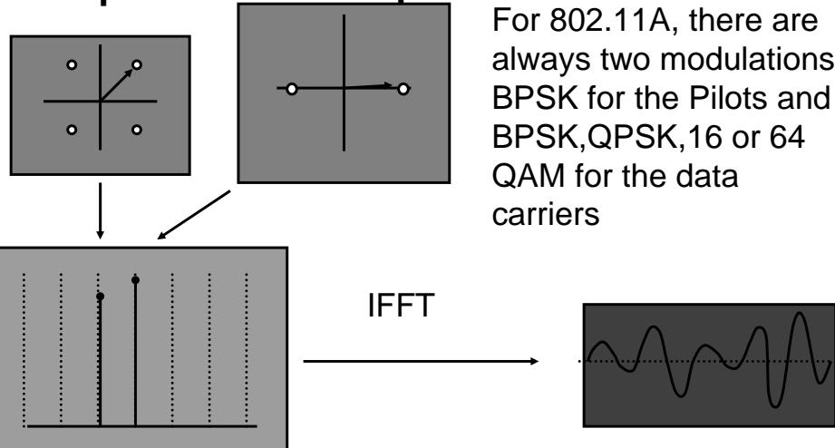
This diagram shows how a multi-carrier OFDM signal is generated, and how easy it is to have many different modulation formats. In the limit, every carrier could be different! As more carriers are added, the resulting time waveform becomes more complex. This is one of the problems with OFDM. As we'll show later, the addition of multiple carriers results in a signal with a high peak-to-average power ratio.
