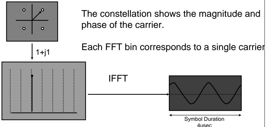
If you know a little about FFT's, the concepts behind OFDM should be very simple to understand. In this example we are going to create an OFDM signal with only one carrier. The magnitude and phase of the carrier are determined from the symbol to be transmitted, as shown in the constellation diagram. The complex number representing the symbol is loaded into an FFT buffer, and an inverse-FFT performed. This produces a set of time-domain samples. These samples are then transmitted.
