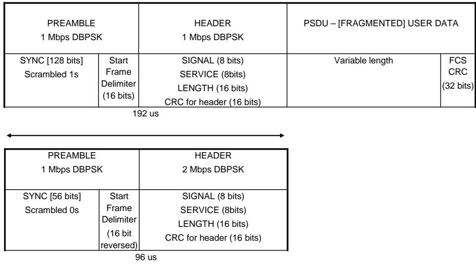
A WLAN device only transmits or receives at one point in time. Transmissions occur as bursts [frames] which vary in length and spacing, usually in the range of a few hundred microseconds to one millisecond. The 802.11b CCA receiver test draws attention to the longest possible 5.5Mbps frame being 3.65ms.
