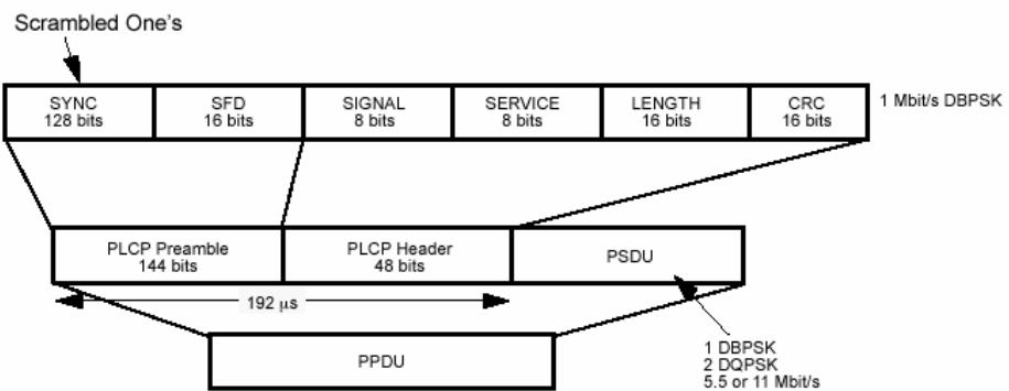
For all 802.11B bit rates, the preamble and header are sent at the 1 Mbit/sec rate. The header is 192 usec long (192 bits). This translates to 2112 chips. The payload data is then appended using one of the four modulation rates
