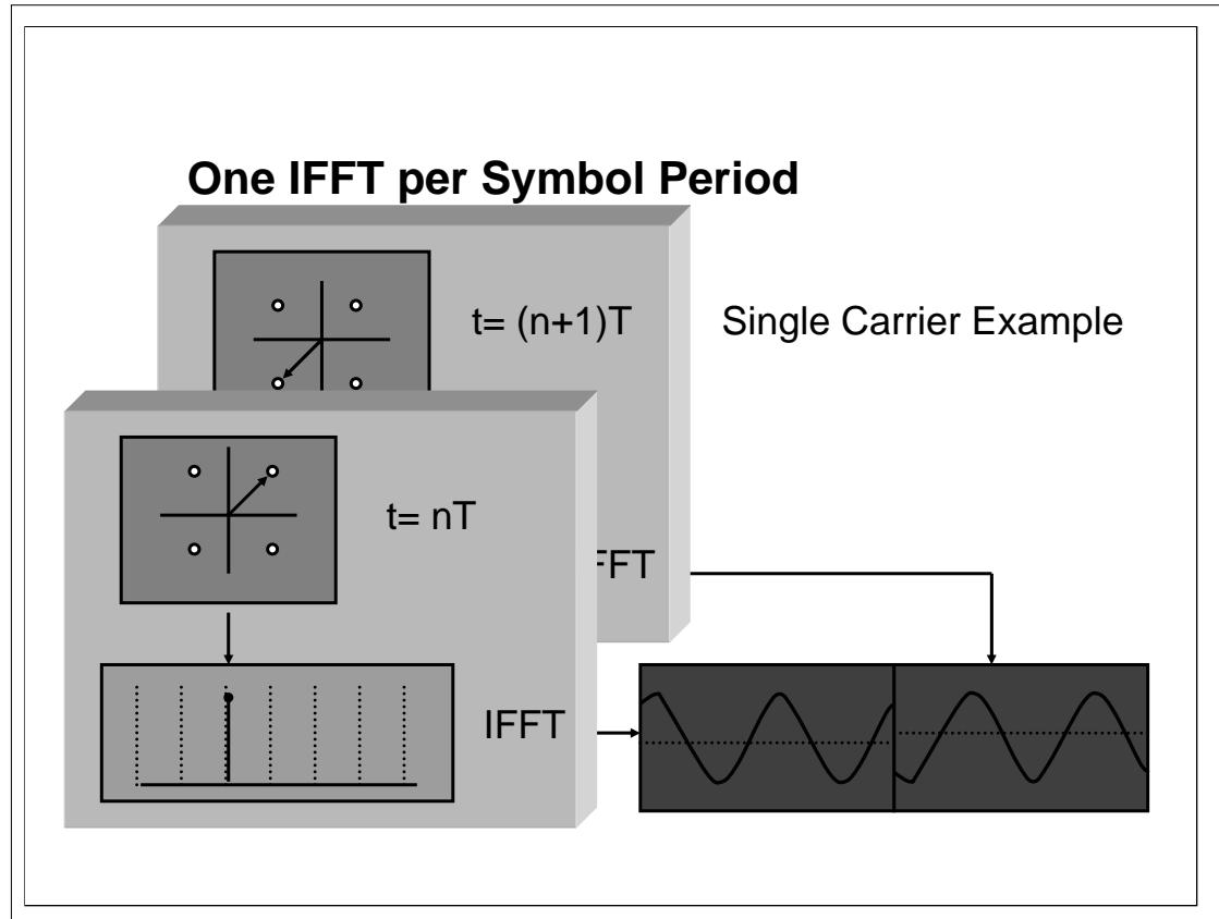
Continuing with the single carrier OFDM example, while the first pulse is being transmitted, the next symbol is loaded into the FFT buffer. Notice that the resulting pulse, when joined with the first, results in a discontinuity. This is normal. The resulting spectral splatter can be attenuated somewhat by windowing the data, as described in the 802.11A standard.
