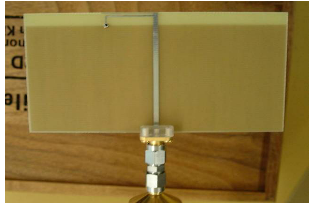
Fig. 17: Measurement setup with antenna on FR-4
