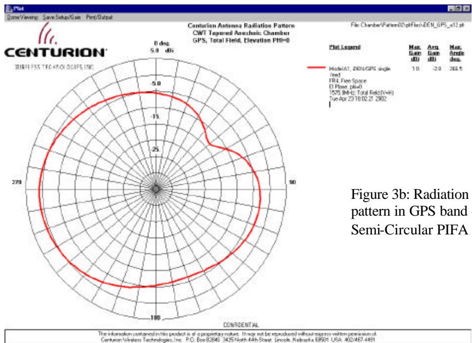
Figure 3b: Radiation pattern in GPS band of Semi-Circular PIFA
