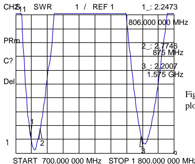
Figure 2: Associated VSWR plot of Semi-Circular PIFA
