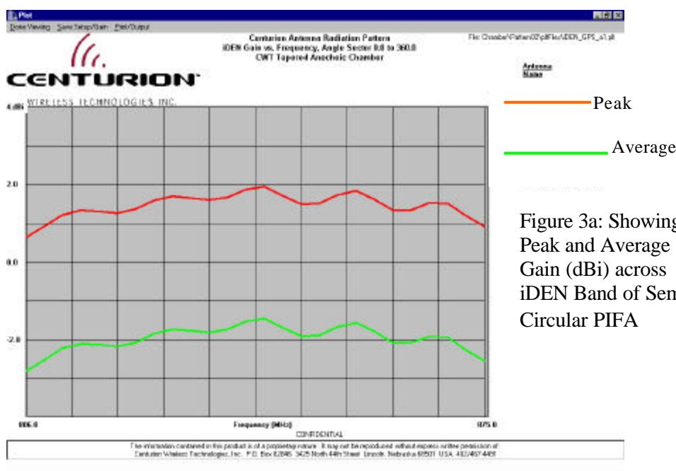
Figure 3a: Showing Peak and Average Gain (dBi) across iDEN Band of Semi-Circular PIFA
