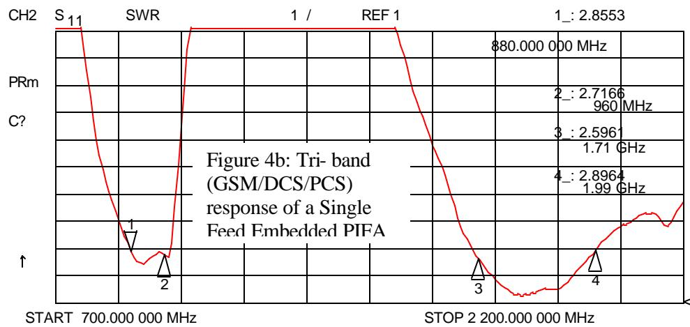
Figure 4b: Tri-band (GSM/DCS/PCS) response of a Single Feed Embedded PIFA
