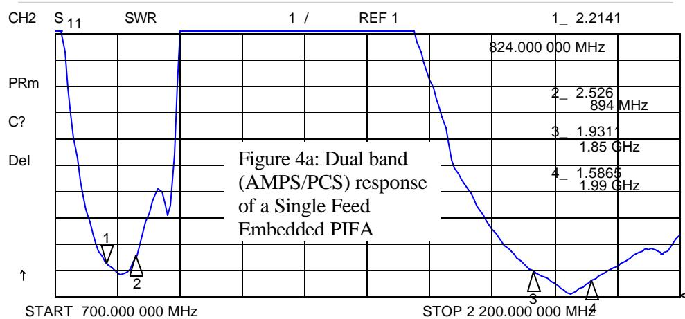
Figure 4a: Dual band (AMPS/PCS) response of a Single Feed Embedded PIFA
