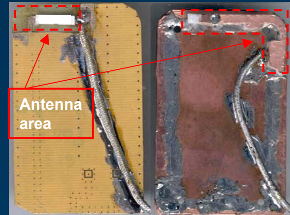
Ceramic chip ant (12x3x2mm)
