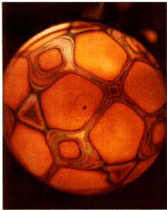
Figure 3. Anisotropic oxidation of a single crystal copper sphere. The fourfold \langle 100 \rangle axis and threefold \langle 111 \rangle axis can be identified. 5
